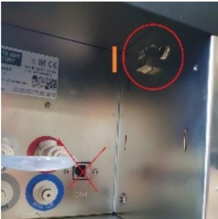
[C] connect the LAN cable from a router to the RJ45 slot (I) on the machine (for LAF BAR see picture from [3.6.2](#))
